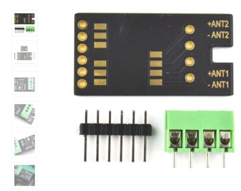
The EverSet ES100-MOD carrier board is a small PCB that breaks out the contacts of the ES100-MOD (castellated holes) to a 6-pin male connector.
